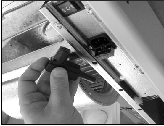
Diagram 5: Mains inlet plug and fuse holder
