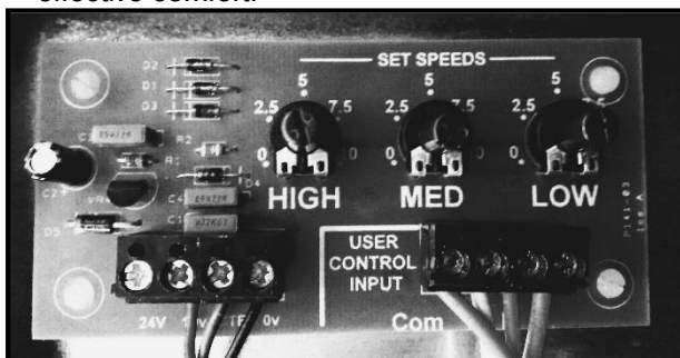
Diagram 8: Fitted 3 speed EC fan controller N.B. All connections are safe low voltage of 10VDC or less.
